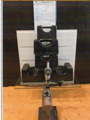
During loading test -NO.1(90kg)
